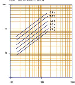
Cross-sectional area of aluminium conductor (mm²)
