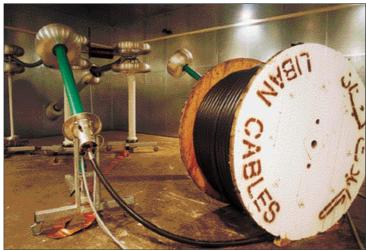
Routine tests and some other tests are carried out in this laboratory. The Faraday cage and its High Voltage transformer provide clearance sufficient for testing reels of cable up to 350 KV.
