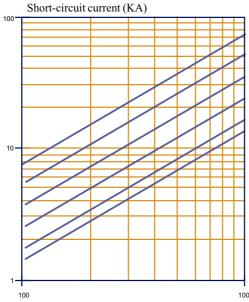
Cross-sectional area of lead screen (mm<sup>2</sup>)
